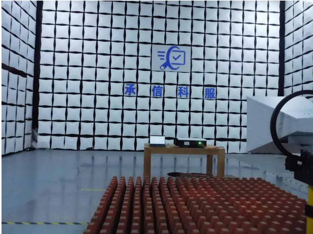
Photograph 4: Set-up for Conducted Susceptibility (CS)
