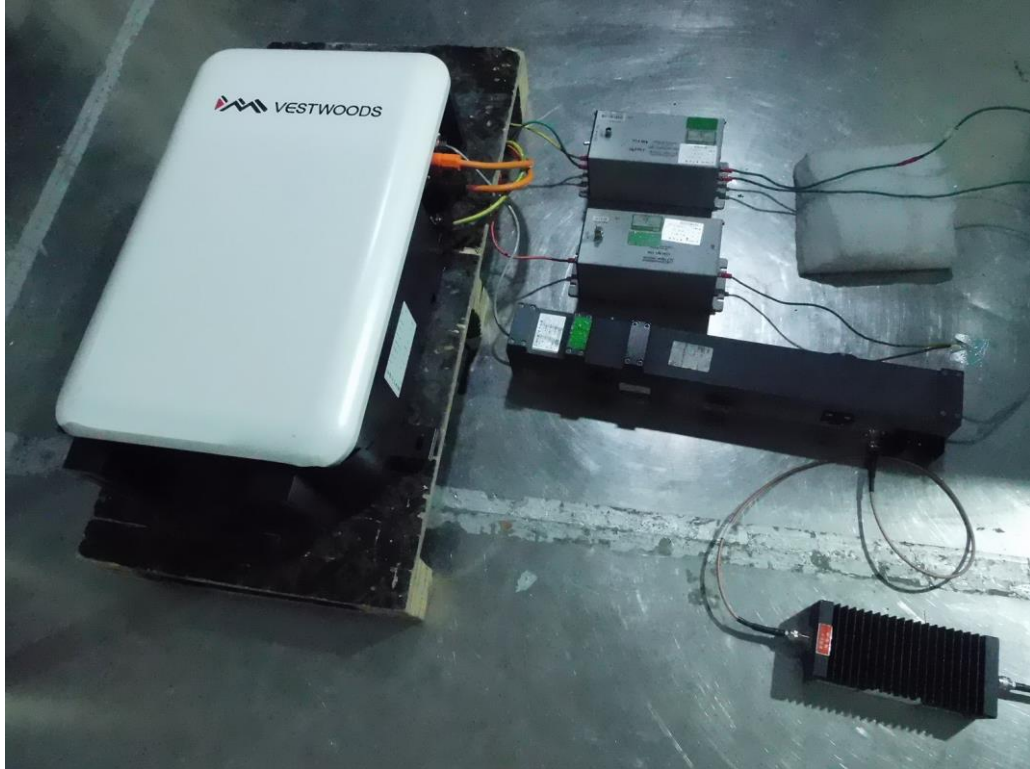
Photograph 5: Set-up for Power-frequency Magnetic Fields
