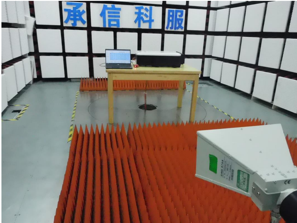
Photograph 3: Set-up for Radio Frequency Electromagnetic Field (RS)
