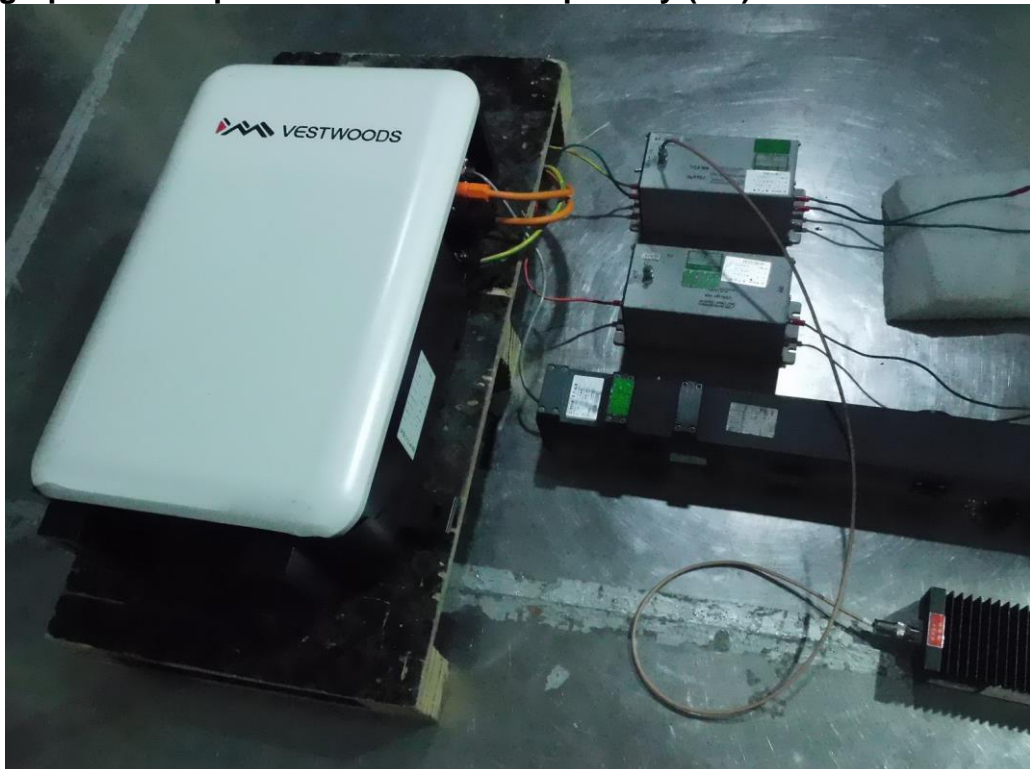
Photograph 4: Set-up for Conducted Susceptibility (CS)
